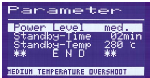
Safe control is possible when temp sensitive components require NO OVERSHOOT! - power level “low”!
