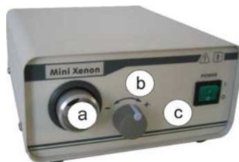
Fig. 2.1 MiniXenon light source
